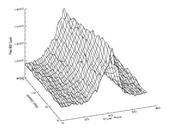
**Fig. 1.** Section of the Darksat trail from the test observation, obtained on 2020/02/08. The section shows a peak pixel count of  $\approx 1600$  and a satellite trail PSF width of 24 pixels. The section is from x(3678:3750), y(1815:1830) of the main FITS.
