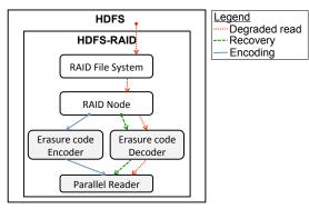
Figure 8: Relevant modules in HDFS-RAID. The execution flow for encoding, degraded reads and reconstruction operations are shown. Hitchhiker is implemented in the shaded modules.
