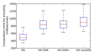
Figure 12: A box plot comparing the computation time for encoding of 1MB (buffer size) from 200 runs each on Facebook's data-warehouse cluster with real-time production traffic and workloads. (HH = Hitchhiker.)
