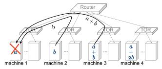
Figure 1: High network usage during reconstruction of erasure-coded data: reconstructing a single missing unit 'a' in this example requires transfer of twice the amount of data through the top-of-rack (TOR) switches.
